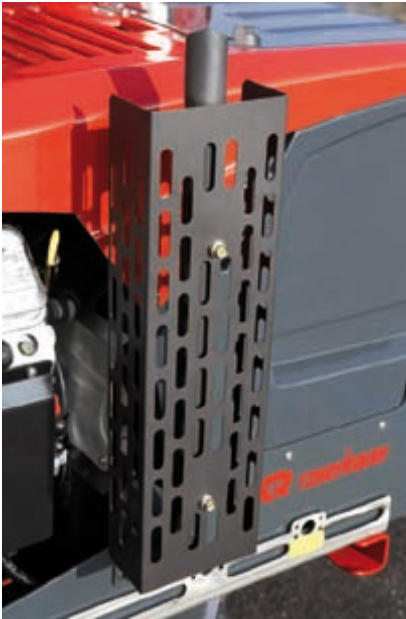
Exhaust gas deflector* for the upward conduction of the gas with turntable ladders
